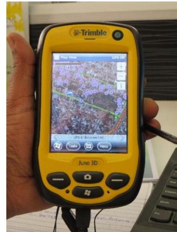
Photo 1 – Hand-held Trimble device to capture points and boundaries
